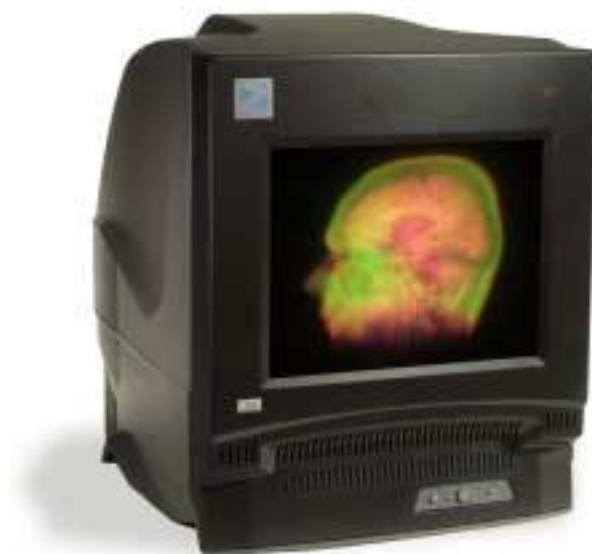
Figure 9.3. Photograph of a commercial DepthCube 3D Display [11]. (Permission for Reprint, courtesy Society for Information Display)
